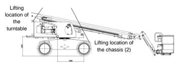
Figure 10-5 Schematic diagram of connection during machine lifting
