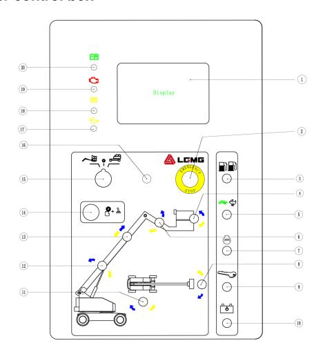
Figure 5-1 Panel of the lower control box
