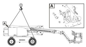
Figure 10-6 Lifting point (take AR20J as an example)
